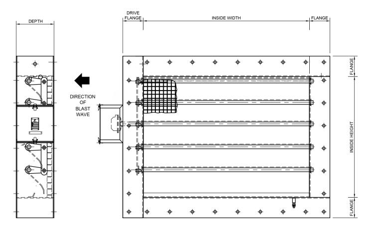
END ELEVATION FRONT ELEVATION
